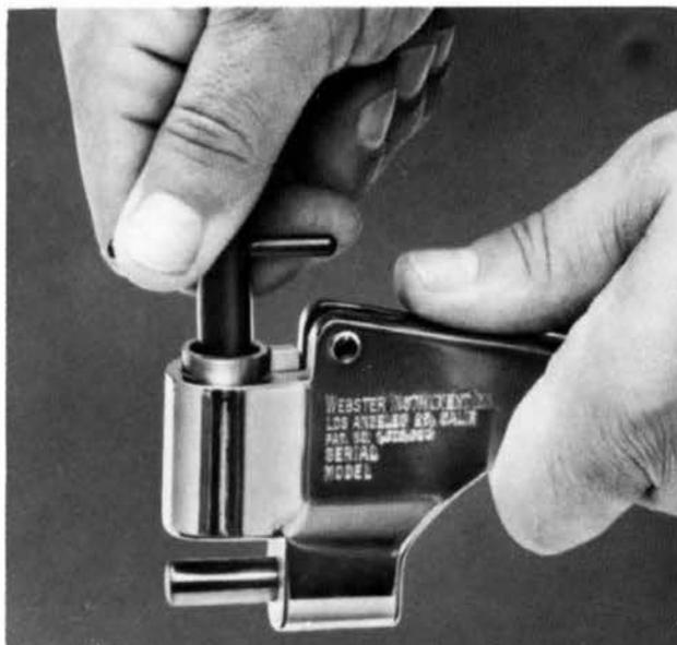
FIG. 4 Adjusting Load on Load Spring
