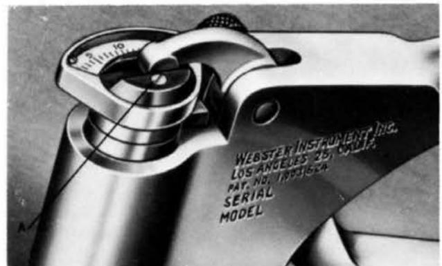
FIG. 3 Zero Adjustment Screw, A (indicated by arrow)
